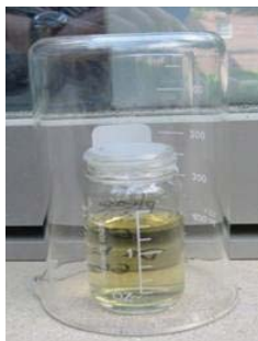
Figure 1 Experimental setup of the study of the effect of sunlight irradiation on the stability of silver nanoparticles.
